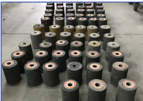
CYLINDRICAL GRINDING STONES FOR TERRAZZO GRINDING MACHINES
